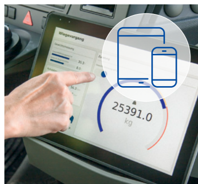
The innovative, calibratable on-board weighing system** determines the payload. It can be operated intuitively either via the screen supplied or via the smartphone using the beSmart app.
