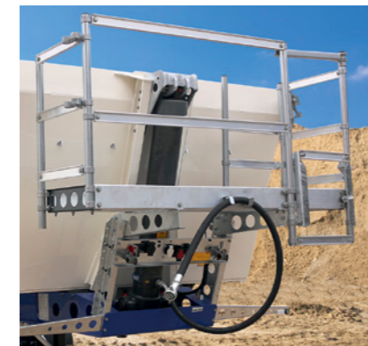
Working platform with improved floor on the tipping trough bulkhead for operation of the rolling tarpaulin. Including trough boarding aid and parking position for the hydraulic hose.
