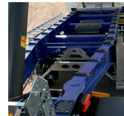
Torsion-resistant steel chassis with improved corrosion protection in painted or galvanised finish with best possible value retention.
