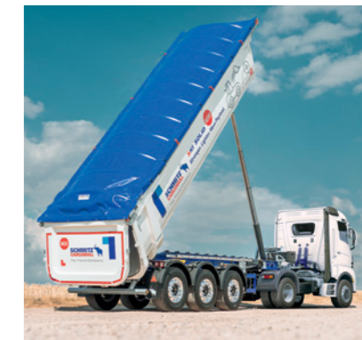
Sliding roof from Schmitz Cargobull enables time-saving opening and closing. Optionally available in manual or electric version, operated by remote control.
