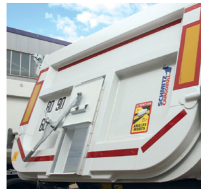
Hydraulic rear wall flap** with automatic function (max. opening cross-section) or can be used as a pendulum flap. Optionally with slide.
