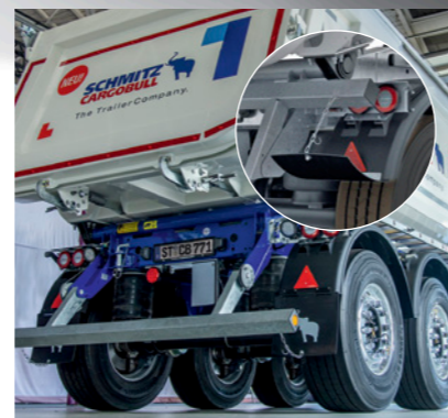
Foldable underride guard with high ground clearance for use on road pavers. Choice of manually operated, supported by spring mechanism or for improved handling in pneumatic version.
